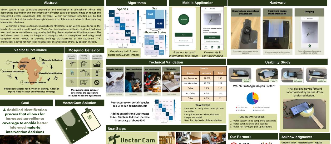
VectorCam is a simple system comprised of two main components: a handheld field tool and mobile phone application that work together to enable automatic mosquito identification
