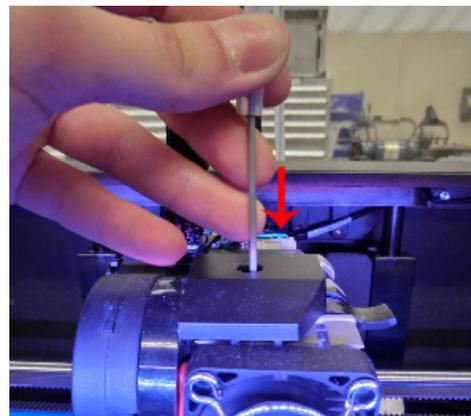
The Makerbot will turn a small motor in the extruder head. Gently feed a small piece of filament sticking out of the clear guide tube into the hole at the top of the extruder head, until the motor catches and begins pulling it down. If the motor does not catch, find a TA or get assistance from a supervisor - do not force the filament in\*. If you are changing colors, you may want to let the extruder purge a few seconds until you have your pure desired color coming out of the extruder.
