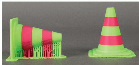
The Makerbot may create a “raft,” a bottom layer designed to be removed underneath your design. Rafts help give parts more stability, especially for parts that are taller than they are wide. Rafts may also help prevent the edges of your part from warping upwards.
