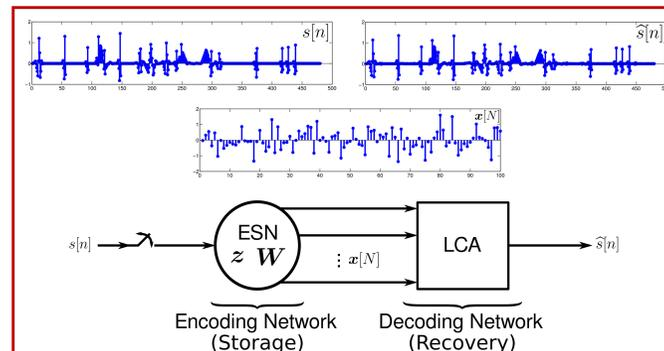
The RIP is satisfied by the ESN for  $N > M$ . Thus, compressible signals are recoverable. Secondary circuits such as the Locally Competitive Algorithm (LCA) could decode the network nodes [9].
